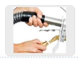
Pull back the smaller brass end of the black solution hose and insert into the connection point under the VAC and PUMP buttons at the front of the machine.
