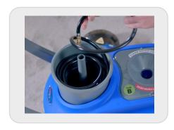
Pull back the brass sleeve on the end of the black solution hose and attach it to the carpet, upholstery or grout & tile wand underneath the trigger until it locks into place.
