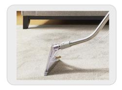
Hold in the spray lever on the wand handle to apply water and solution to the carpet.
