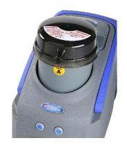
Fill Tank B with 9L of hot water, ensuring the water level does not go above the filter.
